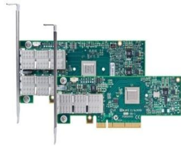
High Performance Interconnects - InfiniBand <1usec latency, 100Gbps Bandwidth>
