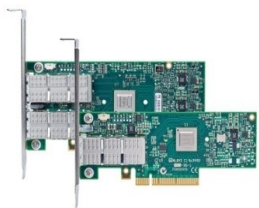
High Performance Interconnects - InfiniBand <1usec latency, 200Gbps Bandwidth>
