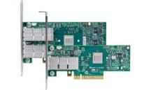
High Performance Interconnects – InfiniBand **(IB),** Omni-Path < 1 μsec latency, 100 Gbps Bandwidth>
