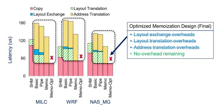
Optimized Memoization design removed all the overheads with zero-copy benefits
