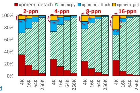
Relative costs of XPMEM API functions for different PPN using one-to-all communication benchmark on a single dual-socket Broadwell node with 14 cores.
