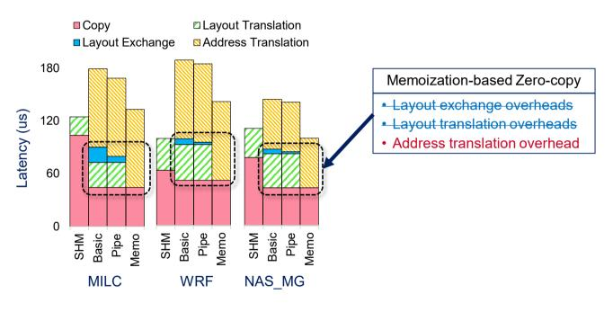
Memoization based design additionally reduced the layout translation overhead
