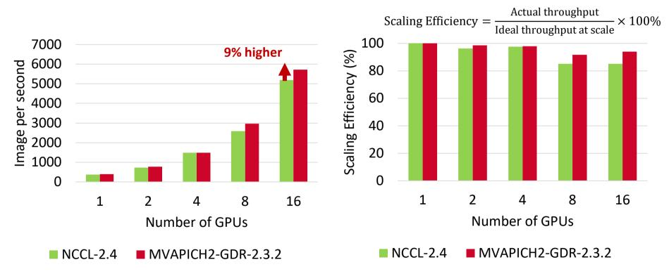
Platform: Nvidia DGX-2 system (16 Nvidia Volta GPUs connected with NVSwitch), CUDA 9.2
